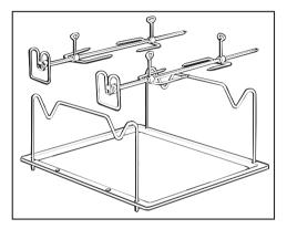
Assemble the rotisserie as shown in the grill pan (with anti-splash tray fitted).
